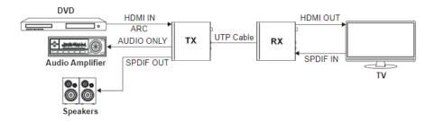
2) Set the Extender to SPDIF Mode. Then switch the LOOP OUT/AUDIO ONLY switch to left, the HDMI OUT port of the transmitter is set to LOOP OUT.
