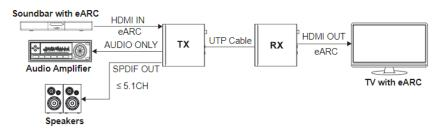
6) Set the Extender to eARC Mode. Then switch the LOOP OUT/AUDIO ONLY switch to left, the HDMI OUT port of the transmitter is set to LOOP OUT.
