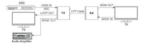
3) Set the Extender to ARC Mode. Then switch the LOOP OUT/AUDIO ONLY switch to right, the HDMI OUT port of the transmitter is set to AUDIO ONLY.
